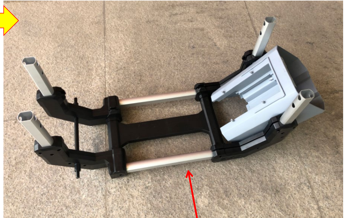
Battery Box & Frame assembly
