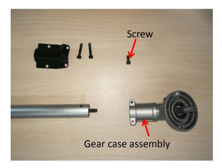
13. Align the hole on the connecting tube with the hole on the gear case and then tighten them together with the screw.
