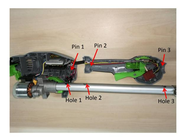
10. Connect connector 1 and tighten the fixed ring with screw.
