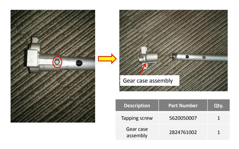
7. Replace the gear case assembly with a new one and assemble the gear case assembly with the shaft assembly with screw.
