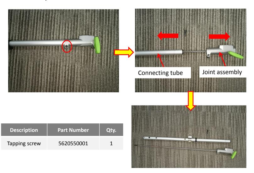
4. Hold the shaft assembly with one hand and pull the joint assembly with the other hand to separate them.
