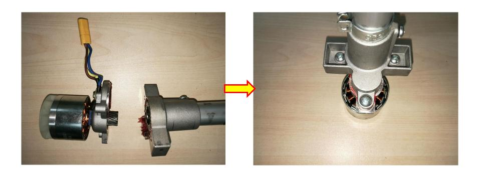
9. Align hole 1 on the shaft assembly with the pin 1 on the left housing assembly , hole 2 with pin 2 and hole 3 with pin 3 separately to mount the motor and shaft assembly onto the housing and handle assembly.
