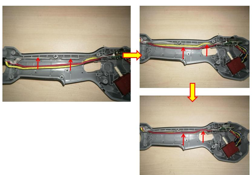
7. Mount the interlock trigger into the groove and lock it with clamp which was tightened by screw, then assemble the switch trigger and speed change button.
