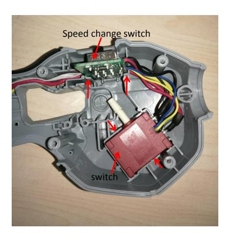
6. Align the white cable, yellow cable and red cable in sequence.
