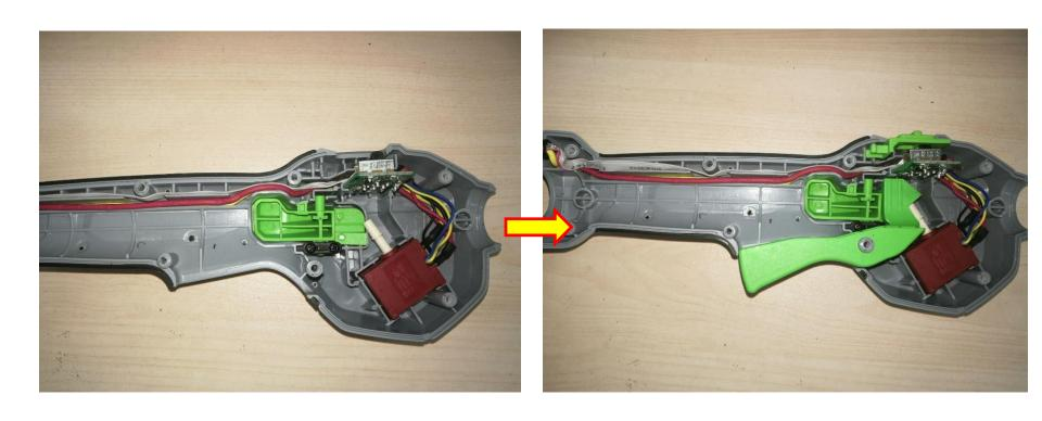
8. Mount the PCB and battery pack connector into the groove and then align the red cable.
