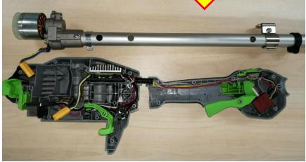
5. Loosen 3 screws to separate the motor from the shaft assembly.
