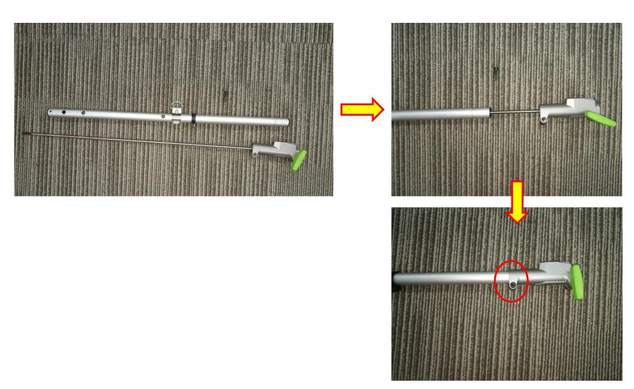
9. Assemble the motor and gear case assembly with shaft assembly with screws.
