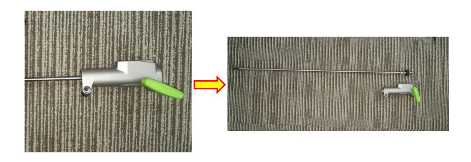
5. Take away the E-ring with circlip plier to separate the bearing wrapped with bearing holder from the shaft assembly.
