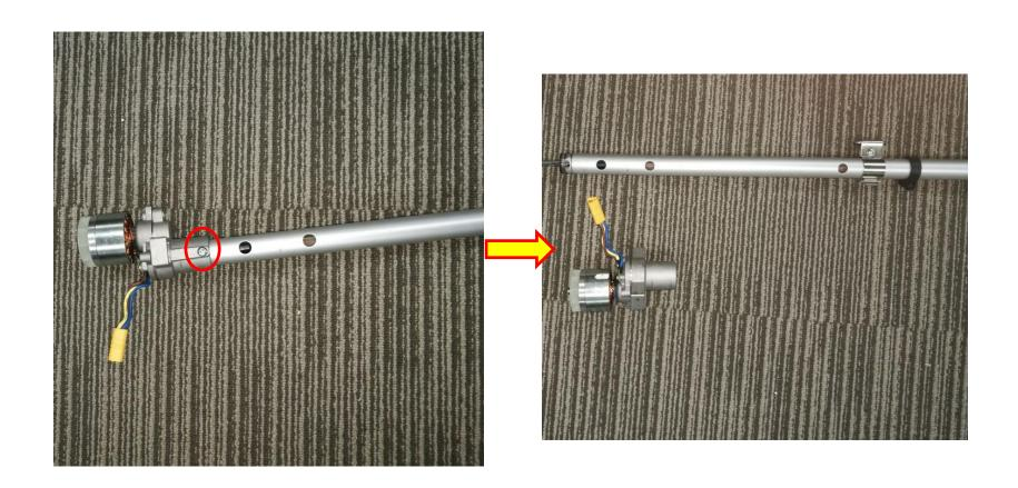
3. Loosen the screw on the joint assembly and pull the connecting tube and joint assembly with each hand to separate them.
