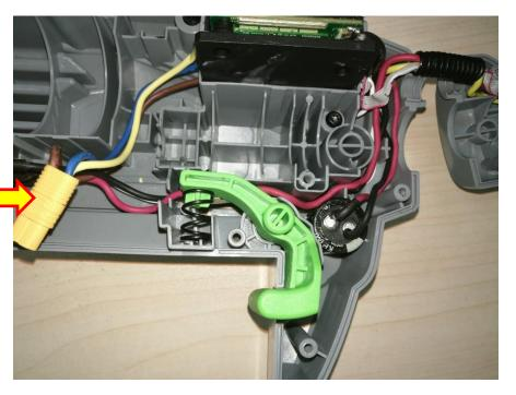
11. Mount the motor and shaft assembly into the housing assembly, connect connector 1 and lock the fixed ring with screw, then assemble the handle assembly as shown in the "Replace the Motor Assembly" section.
