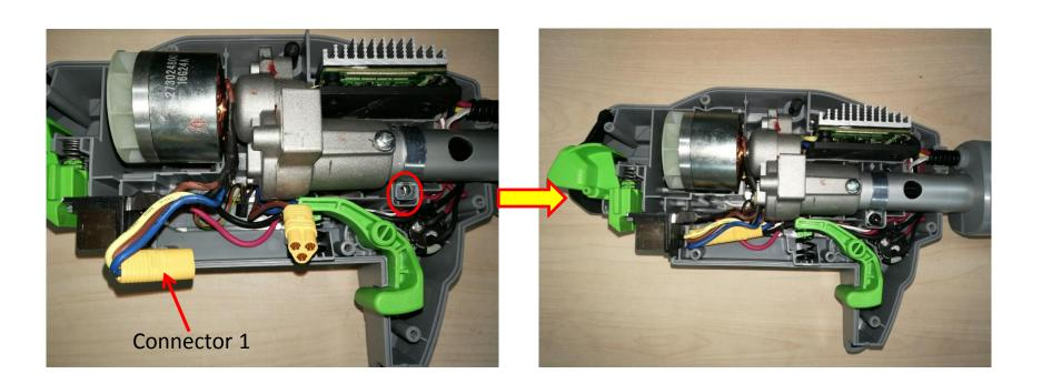
11. Assemble the handle housing assembly with screws.
