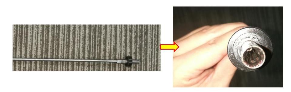
7. Insert the side with bearing of the shaft assembly into the joint assembly
