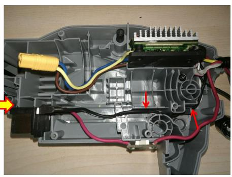
9. Align the red cable, then mount the capacitor into the groove and align the black and white cables into the groove.
