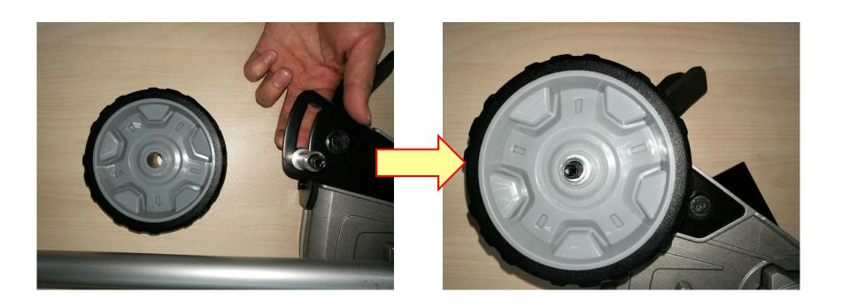
11. Mount plain washer 2 and spring washer onto the pole screw in sequence.
