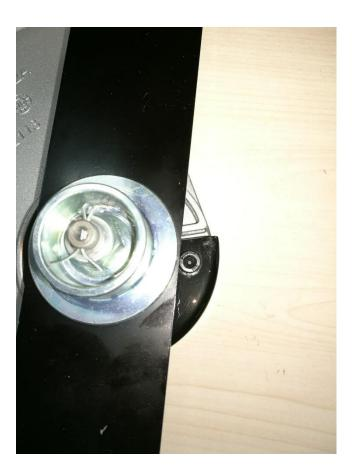
5. Assemble the guide plate with the anti-wear protective guard with screw.
