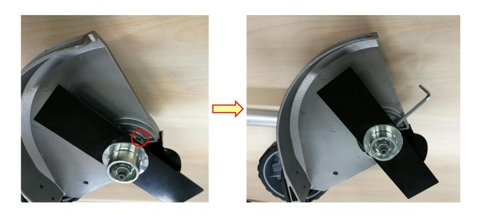
4. Loosen the nut clockwise with the multifunction wrench to remove it.
