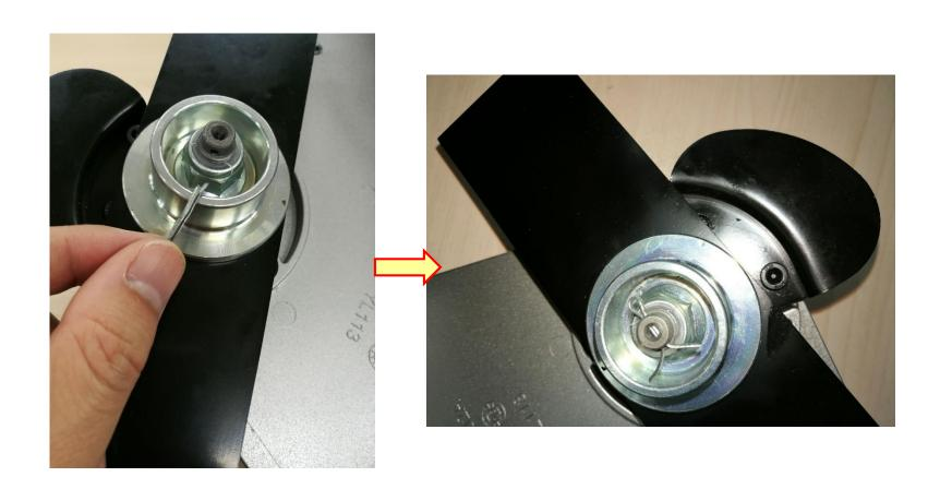
1. Loosen the screw on the guide plate to remove it.
