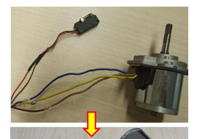
Measure the resistance between any of the two terminals
