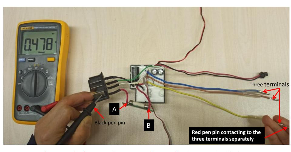
**NOTICE:** in this step, the fuse must be measured as good. Otherwise, the black pen pin should be contacted to "B", rather than "A" (the battery electric contact that is connected to the red cable side), before having fuse final measurement.
