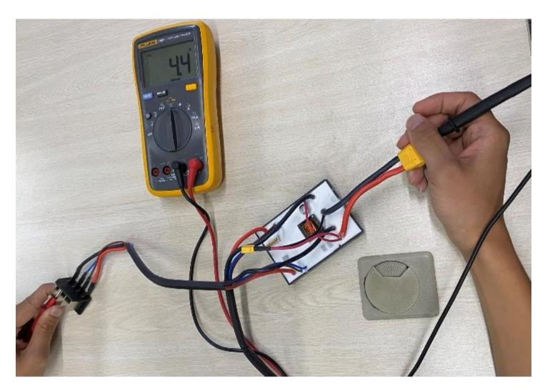
**NOTICE:** The same measurement for the other contact of the battery pack due to the snow blower is equipped with two battery compartments.
