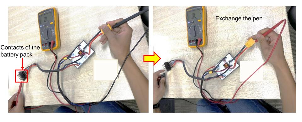
**NOTICE:** The same measurements for the other contact of the battery pack due to the snow blower is equipped with two battery compartments.
