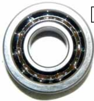
Bearing side towards the outside of the shaft
